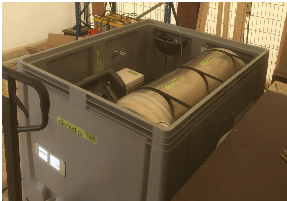
Figure 8. The Diamedica prototype low-pressure oxygen system. The top of the oxygen concentrator can be seen to the left and the upper of the two storage vessels at the right. In the pallet box, the compressor is also installed. The prototype further contains a unit for handling varying quality grid power or 12 V solar power direct input – but these features were not used in the current tests.
